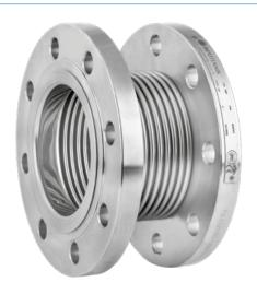
This type of expansion joints are also called as "Vanstone" or "floating flange" type. Flanges are not welded to a bellows or pipe, they simply rotate over the bellows "neck" or pipe. Suitable for lower pressures, carbon steel flanges can be used at internally corrosive environments since the bellows material separates the flanges from internal medium. Rotating flanges eliminates the problem of flange bolt misalignment during installation.
