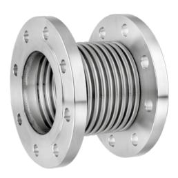
These units come with welded flanges on both ends. This type of assembly provides easy connection in the field (no welding required), easy replacement and can be used at high pressures. Flanges can be manufactured from carbon steel, stainless steel or nickel alloys conforming to many industry standards such as ASME, EN, JIS, etc.
